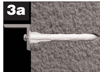
3a Anti-rotation fins prevent spinning while the ALLIGATOR anchor expands along the screw in solid walls ... up to 2x its original length.
